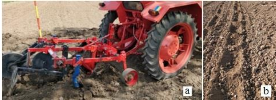
Fig. 1. Experimental activity: a –working aggregate; b – channels and dams generated
