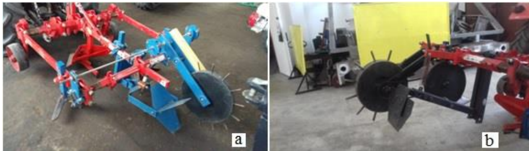
Fig. 2. Rotor version of the EOCFW load-bearing structure (a), and the cam version, (b)
